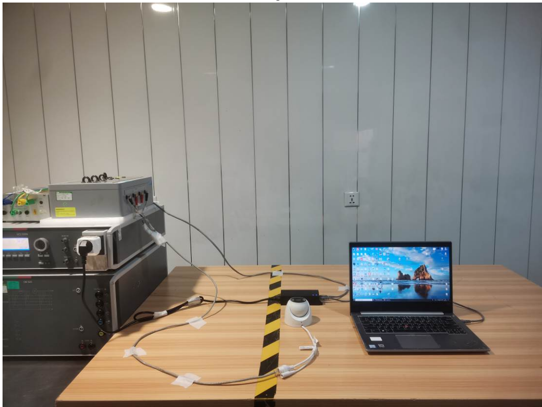
PoE Port Test Setup Photo View-M2
