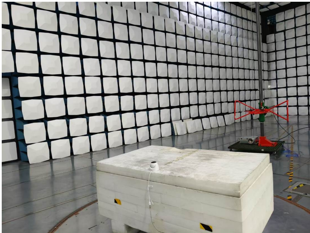
Radiated Emissions Below 1GHz rear View-M2
