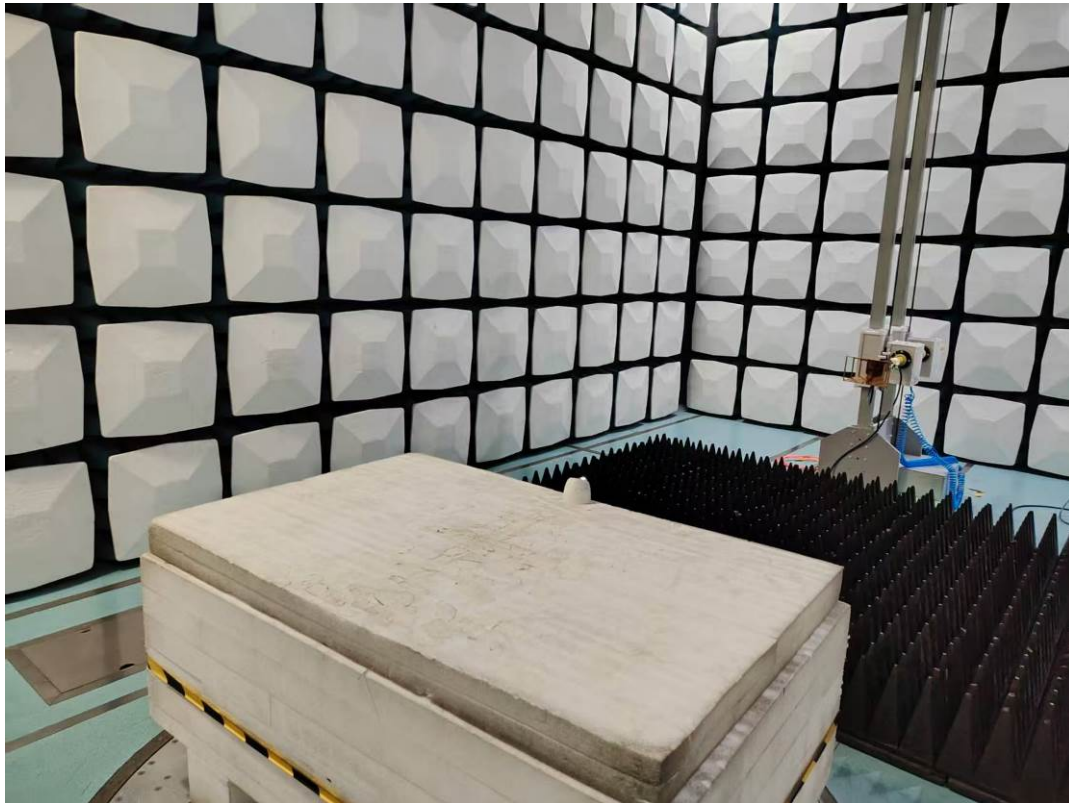
Radiated Emissions Above 1GHz rear View-M2
